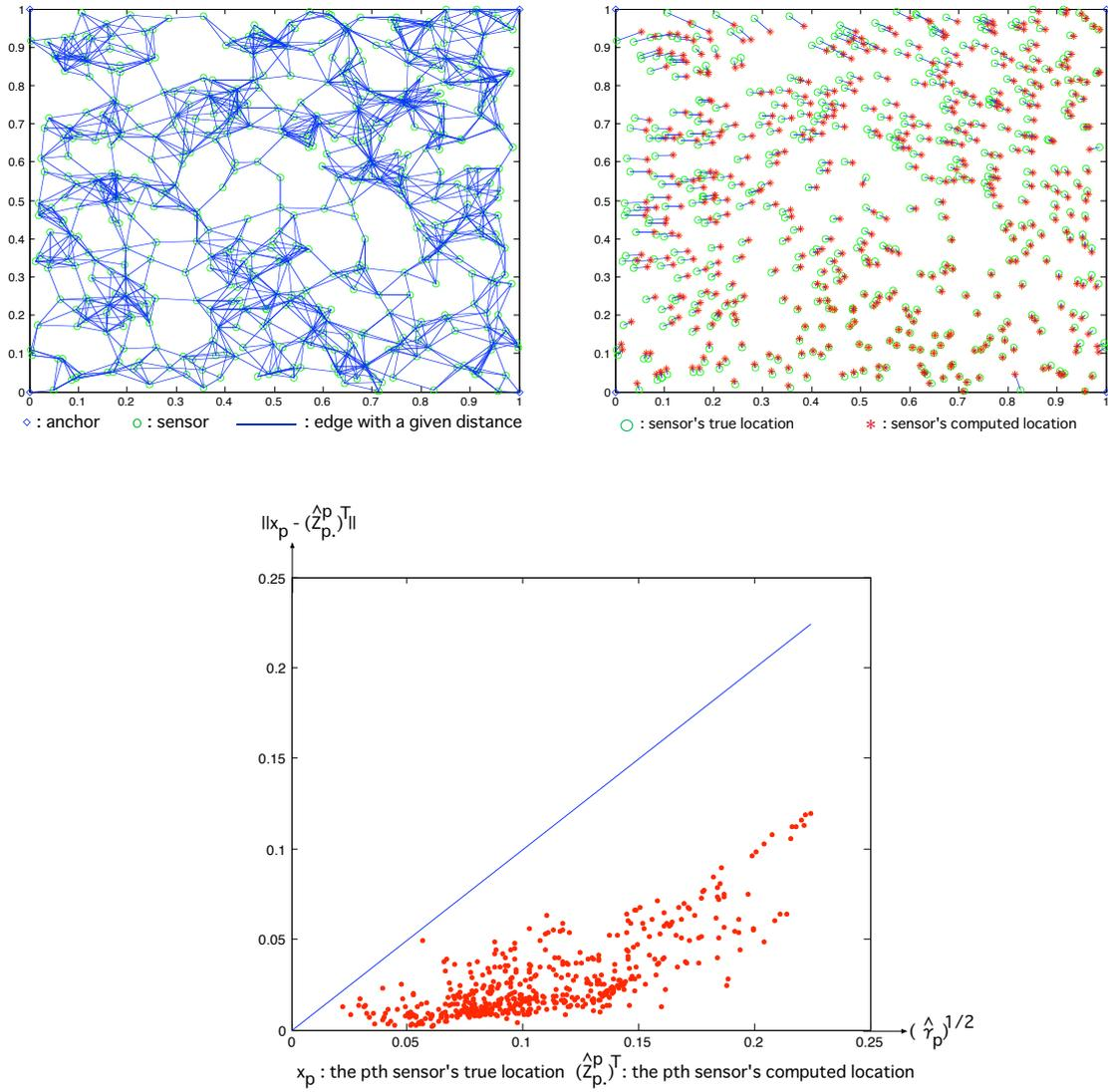
Figure 2: A 2-dimensional sensor network localization problem with randomly distributed 500 sensors in  $[0, 1] \times [0, 1]$ , 4 anchors at the corner and  $\rho = 0.09$ .
